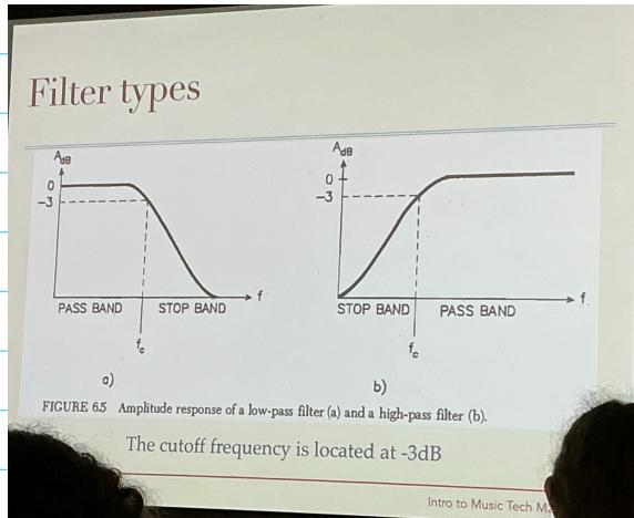
FIGURE 6.5 Amplitude response of a low-pass filter (a) and a high-pass filter (b).
